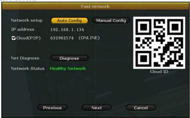
[Network Setup]: Two ways, Auto Config and Manual Config. [Cloud(P2P)]: The code is used to add the device to the P2P account.
