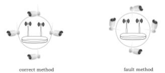
The signal coverage of Antenna is similar to a round circle. Antenna located in
